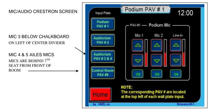
MIC 3 VOLUME CONTROL CRESTRON SCREEN (MIC CONNECTOR IS BELOW CHALKBOARD TO THE LEFT OF THE CENTER CHALKBOARD DEVIDER)
