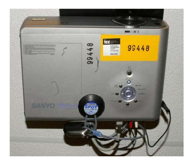
Projectors and plasma and LCD screens are to be tagged and registered with the STOP system. Installer must also secure document cameras to the podium using Securtech security cable, puck and padlock supplied by NCS
